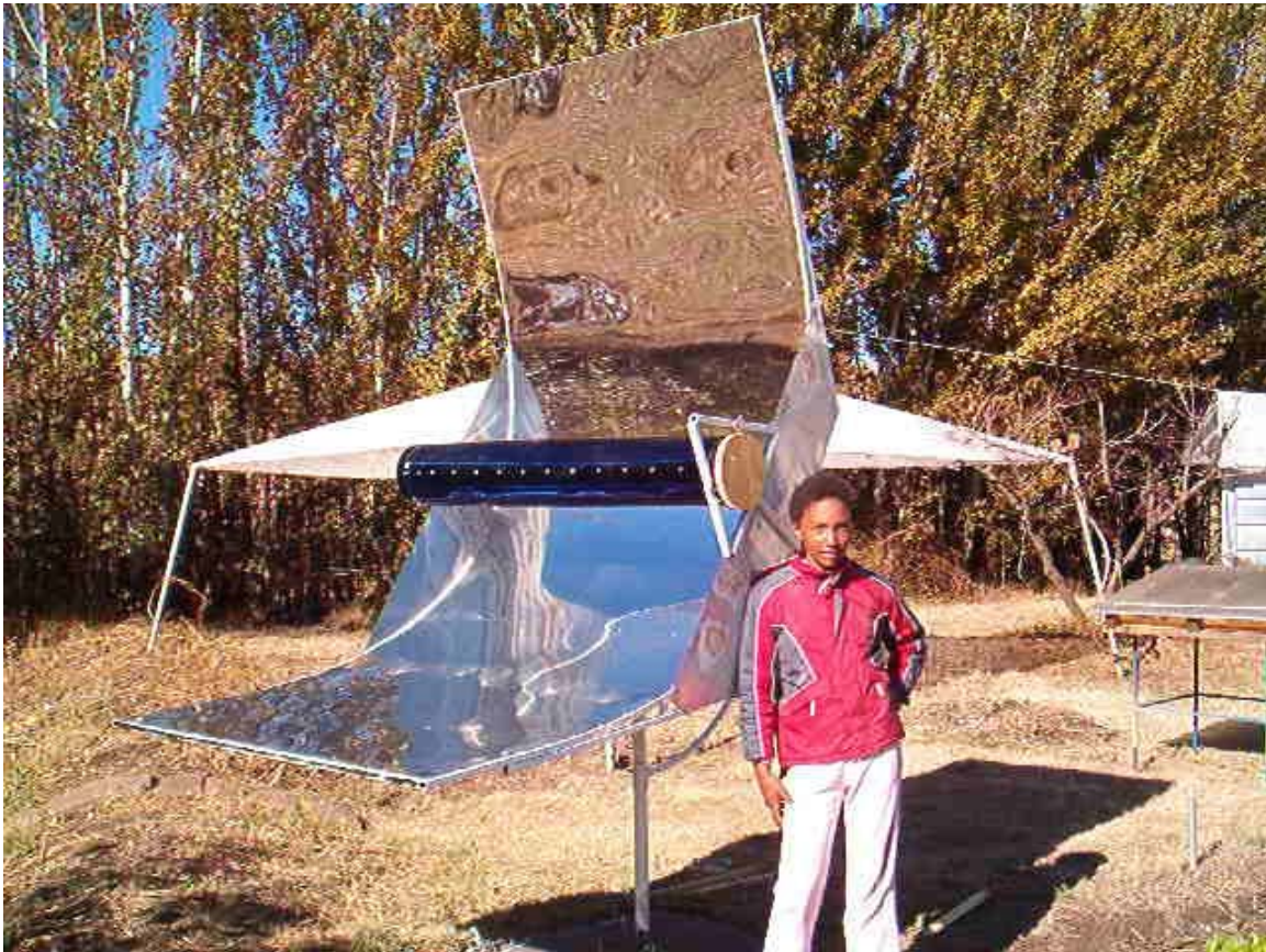
Fig. 1: Front view of concentrator type baking device. Author's daughter Thung-Thung in foreground. Absorber tube is loaded/unloaded by removing plywood plug on end.
